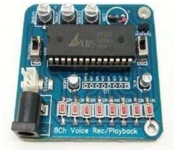
Fig 3.13: APR33A3 Voice Playback Module
